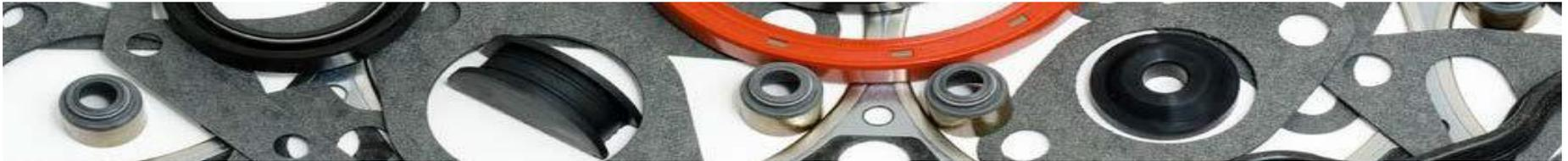
Equipment and piping must be able to keep in, or out, critical process fluids and hazardous gases to operate safely and efficiently. Seals, including gaskets and packing, fill the role for a variety of applications. The *Static and Dynamic Sealing* subject area covers not only seals, but also common methods of connecting equipment and piping.
