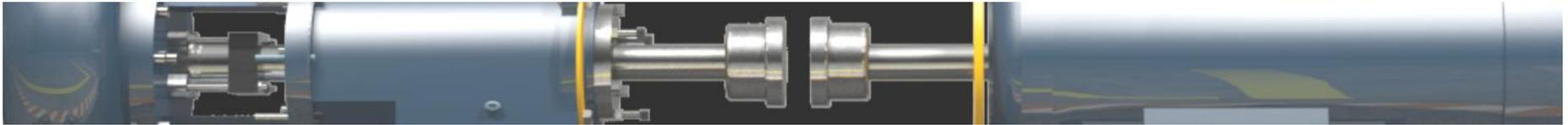
It's estimated that 50–70% of all vibration problems in machines are caused by shaft misalignment. This series, *Shaft Alignment*, address the types and effects of this common problem, along with methods to correct it. The emergence of new technologies has improved shaft alignment procedures, which is also covered in this subject area.
