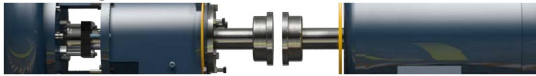
It's estimated that 50-70% of all vibration problems in machines are caused by shaft misalignment. This series of modules, Shaft Alignment, will address the types and effects of this common problem, along with methods to correct it. The emergence of new technologies has improved shaft alignment procedures, which is also covered in this subject area.
