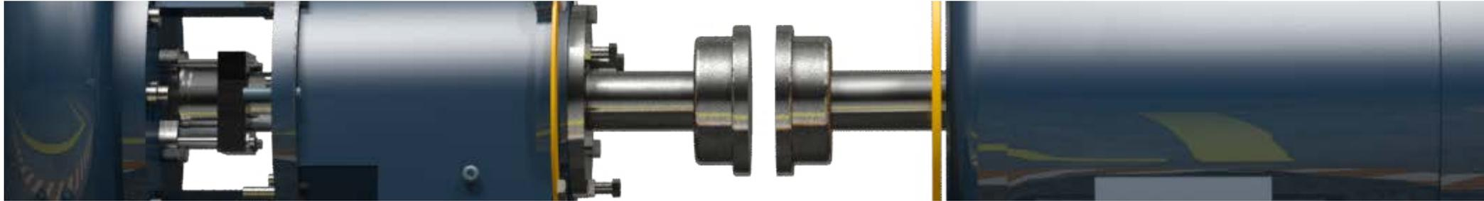
It's estimated that 50 – 70% of all vibration problems in machines are caused by shaft misalignment. This series of modules, Shaft Alignment, will address the types and effects of this common problem, along with methods to correct it. The emergence of new technologies has improved shaft alignment procedures, which is also covered in this subject area.
