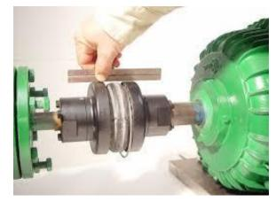
This three-day course introduces the principles of power transmission couplings and shaft alignment. Next, the various types and purposes of couplings are discussed. Alignment processes are introduced followed by practical, hands-on exercises. Finally, methods of measuring misalignment in rotating machinery conclude the course. This course is ideal for plant personnel responsible for the installation, operation, maintenance, and reliability of rotating equipment fitted with couplings.
